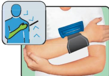
5. The positioning system shown on the left and a beep confirm that you have reached the right measuring position. The measurement will start automatically.
